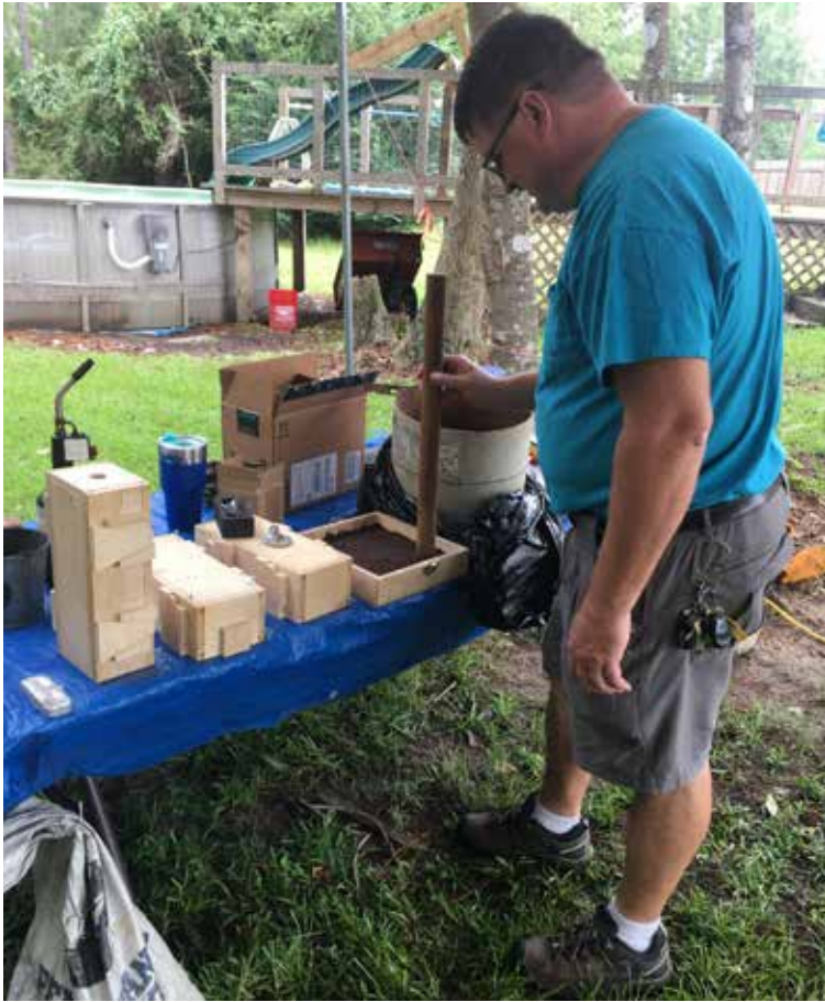
John Butler packing the sand into the drag.
