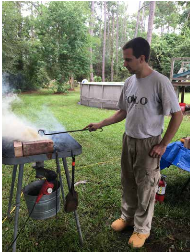
Christopher Sandlin attending to the melting of the aluminum. This batch of metal had zinc in it and had to be abandoned.
