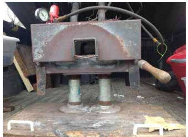
Above is my propane forge. More wood and pipe collars. The handles are used to slide it in and out of truck bed. Note the charred wood. I use a split #10 Can to shield wood. A metal base plate to start with might have been better.
