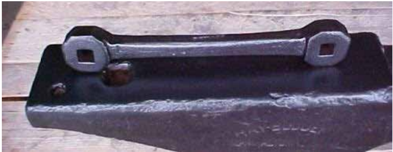
Example of a square bolt header. They were once made for six-sided bolts, too. (Photo credit Etsy)
