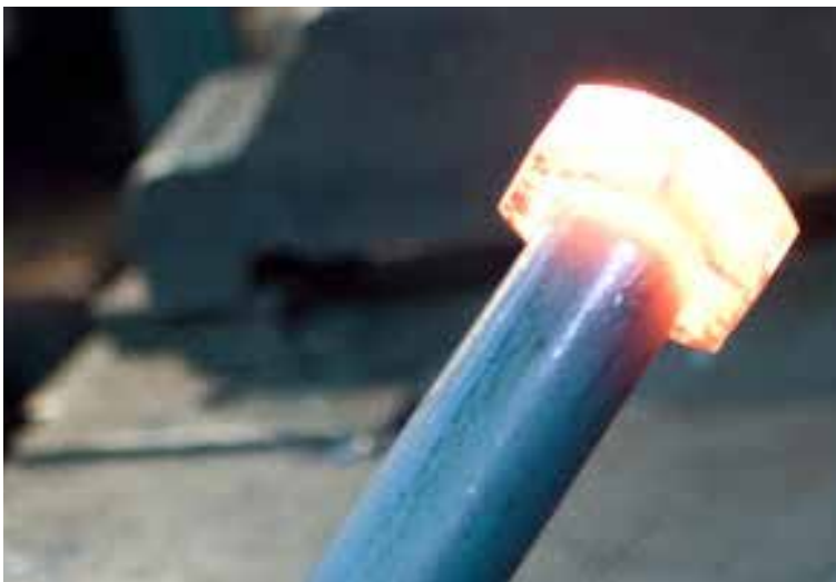
Ring wrapped, forge welded and shaped around a rod to make a bolt head (photo credit, Portland Bolt)
