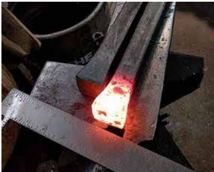
Example of a short heat for upsetting iron (Photo credit Javos Ironworks)
