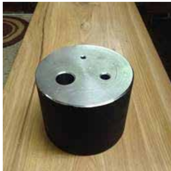
Example of a "monkey tool", some are single size, many have handles. (Photo credit Anvil Fire discussion board)
