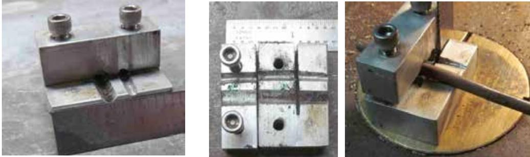
Start with 1.5" x 1.5" x 0.5" aluminum bar (or 1.5" x 1" x 0.5" & 0.5" x 0.5" x 1.5" if you want to avoid a saw cut). You will need to have access to a mill or a drill press with a cross-slide vise and a 2-flute end mill (1/4" diameter or thereabouts).
