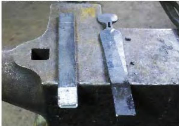
The one pictured has been slot punched for a thumb latch, but this is not necessary for a regular pull. Next, turn the piece around and fuller at the mark on the other end. Start to taper the body of the piece down to the fuller, being careful of the bevel you have made. Once this looks good, bevel out the beam on this end to match the first one. See photo two.
