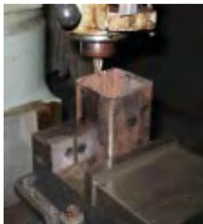
The tuyere downpipe was mild steel 5" long x 3" square (1/8" wall) and I got to use my new toy - a Bridgeport clone - to mill the ends square and flat. The horizontal section was a 4" of 3" diameter black pipe. The pipe was cut with a Rigid pipe cutter, so squaring wasn't needed.
