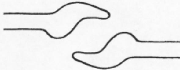
2. Shape ends so they will 'scarf' together. Scarf should be thin but not too thin.
