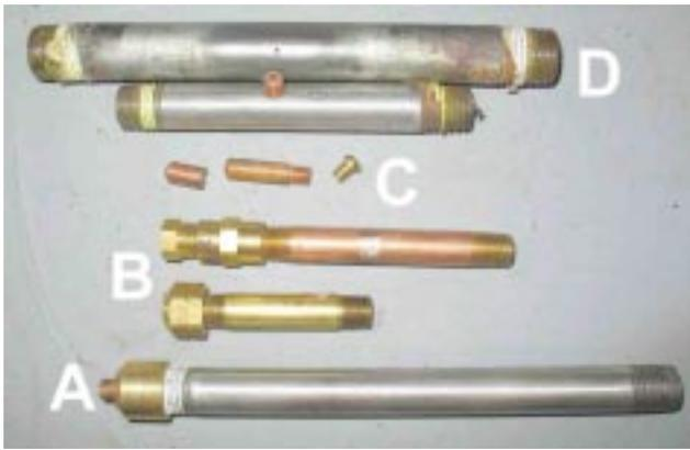
Figure 9: Gas delivery tubes
