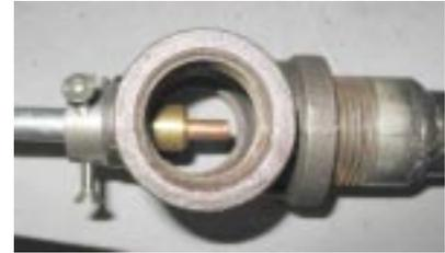
Figure 15: A “T” burner with tip 1” from junction
