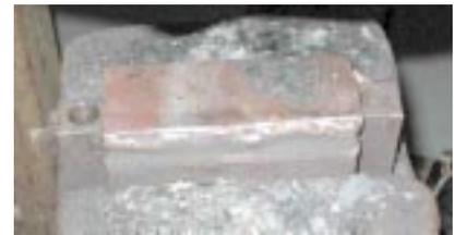
Figure 4: Lower die with hardy holes
