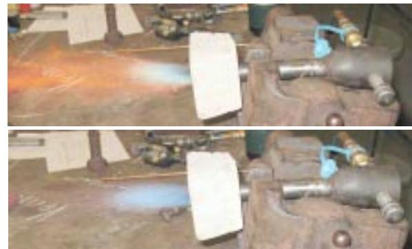
Figure 11: Tuning a bell burner
