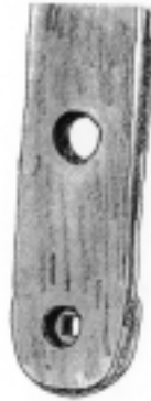
Backside of Header, note the relief drill in the backer bar. The other hole is for hanging.
