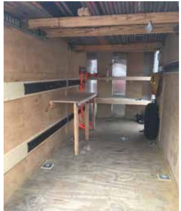
Floor and wall anchor systems in place, overhead storage of the tent poles, shelving with moveable legs to hold tents, tools and gas forges.
