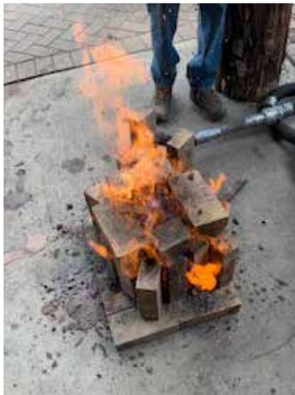
the Viking foundry. Also like the Viking foundry the ore is added just opposite the center line away from the twyer with a minor difference in that the majority of the ore is placed toward the center and allowed to taper out to the sides, otherwise everything else was run the same as the short stack.
