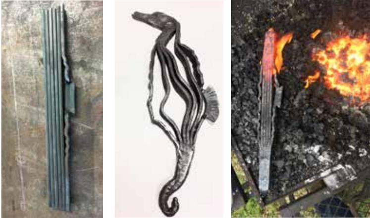
Tony Fenn made a Seahorse using six 14-inch long pieces of 1/4 inch by 1/4 inch. These were forge welded at each end, then heated in the middle and hammered in the vice to open up the body. The head and tail were then forged to complete the piece.
