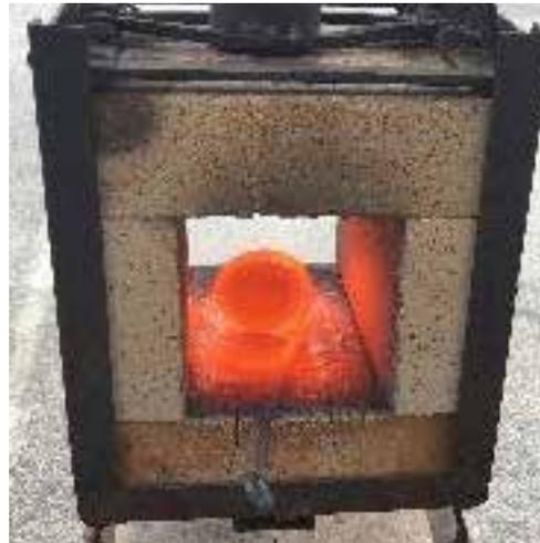
Steps in pulling out the basket: Heat the coil evenly, then quench the hanging bar so it won't bend as you pull. An even pull straight up will do the trick.
