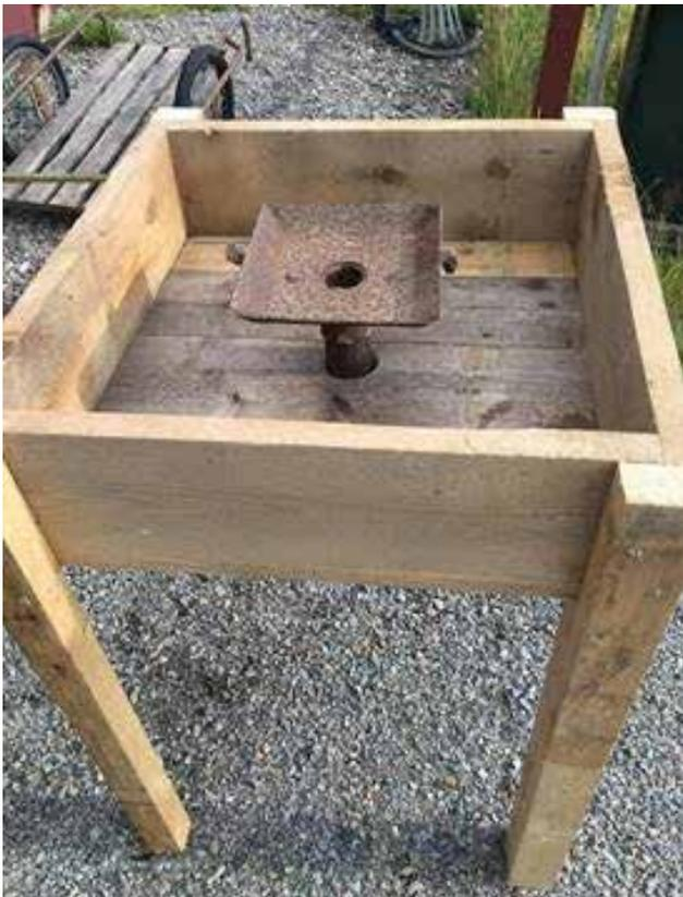
Dirt box forge, prior to putting the dirt in. Note the only available pan was about 1" deep so dirt will make up part of the pot.
