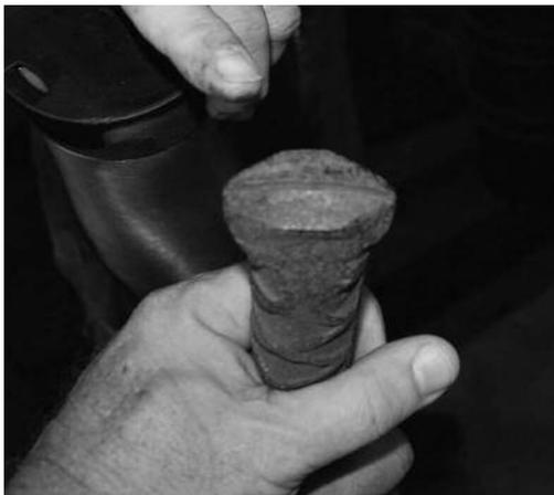
repetitively hammer the hot end while holding the bar in your hand, try hammering the bar while using your hand to push the bar against the hammer hard.
