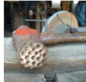
hammering a piece of 3/4" Shld 40 black steel pipe on the point the horn and on the anvil face to flatten the flair. Jerry used a Guillotine fuller to crimp the pipe down to about a 1/4" diameter. He cuts the cup off, threads the bottom of the cup and bolts it to the base.
