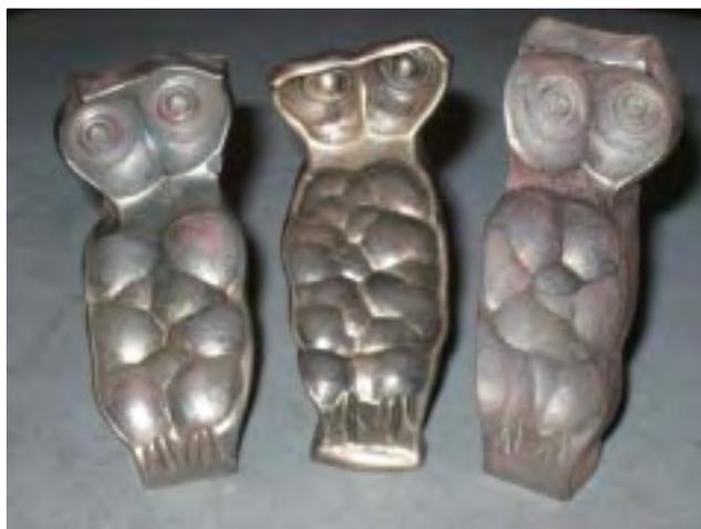
Then the outer portion of the punch is ground away to give a punch with a "thin edge" (approximately 1/16" or less) around the ball impression. Since S-7 is air hardening, it is ready to go. The owl eye sockets are made using a ball peen hammer and the feathery body appearance is created by overlapping ball peen indentations.
