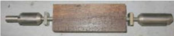
the block is ready and the spacers cut from flat stock, the pieces are assembled on the mandrel pictures above - basically a piece of 1/4x20 all-thread and two threaded pieces of round stock. One end is set up to accept a live center and the other goes into the three-jaw chuck on my lathe. In place, it looks
