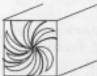
The bar is then squared up again using stop plates on the hammer dies to keep the bar uniform. Again, 3/8" x 3/8" x ?-long.
