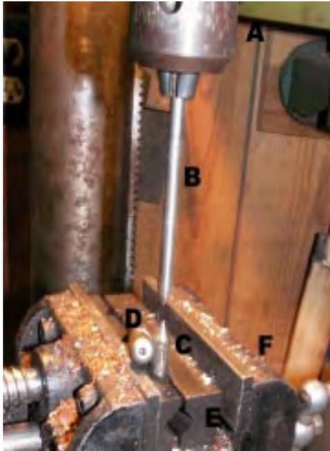
Fig.13: Boring holes through handles
