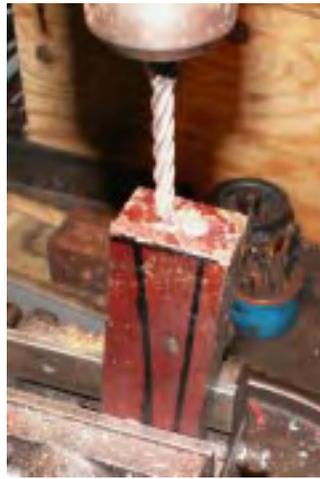
Fig.17: Drill flanking holes
