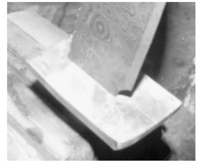
**Fig.8: Guard ready for soldering**
