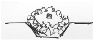
Instead, pack the coke coals closely around the workpiece. Direct contact transfer more heat. But you also run the risk of clinker & green coal sticking to it, so keep your fire well tended.
