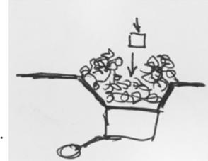
Resting the work piece in a "cave" only warms it & will not get it to the proper welding temperature
